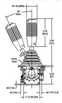
CS1 with an RHS rocker handle and internal potentiometer
