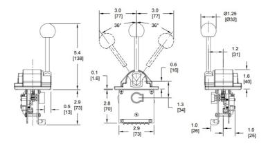
PRO-5 dimensions with round ball handle and potentiometer board.
